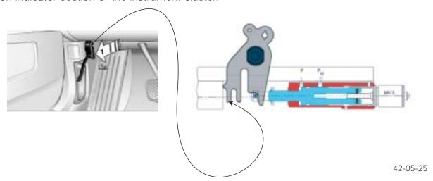
The emergency release must be reset to re-engage the parking lock after eliminating the fault. The gearbox lever moves during normal operation and must not be influenced by the cable assembly. Press on the red tab on the back side of the lever and guide the lever assembly back into the original position.
